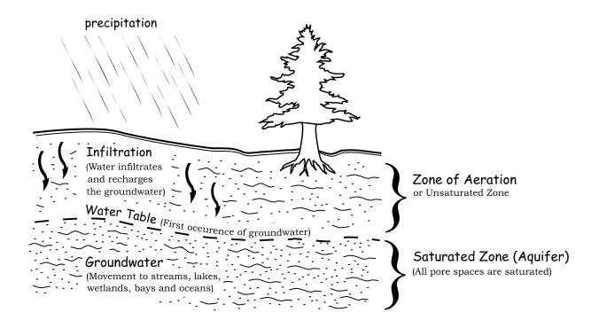
Aquifers are geologic formations – layers of sand, gravel and rock – where significant amounts of water can be stored, transported or supplied to well or a spring. They are irregular in shape, and can be close to the surface, or very deep. Under your home, there may be several aquifers layered one on top of another. Because of this, neighboring homes potentially can have their wells in different aquifers and experience different water quality.
